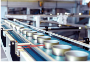
Confirm the passage of cans on the conveyor belt
