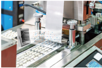
Static elimination during blister packaging
